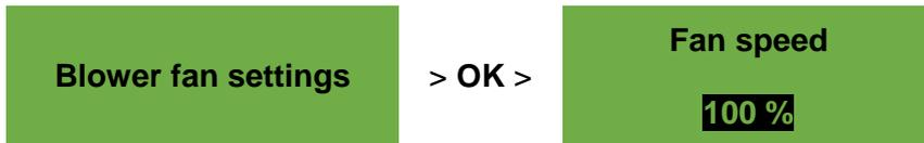
Correct the fan speed in 1% increments using the plus/minus buttons until the desired fan speed is set.
