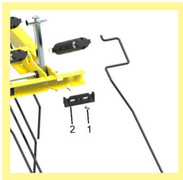
Figure 15: 1 = nut, 2 = plastic piece
